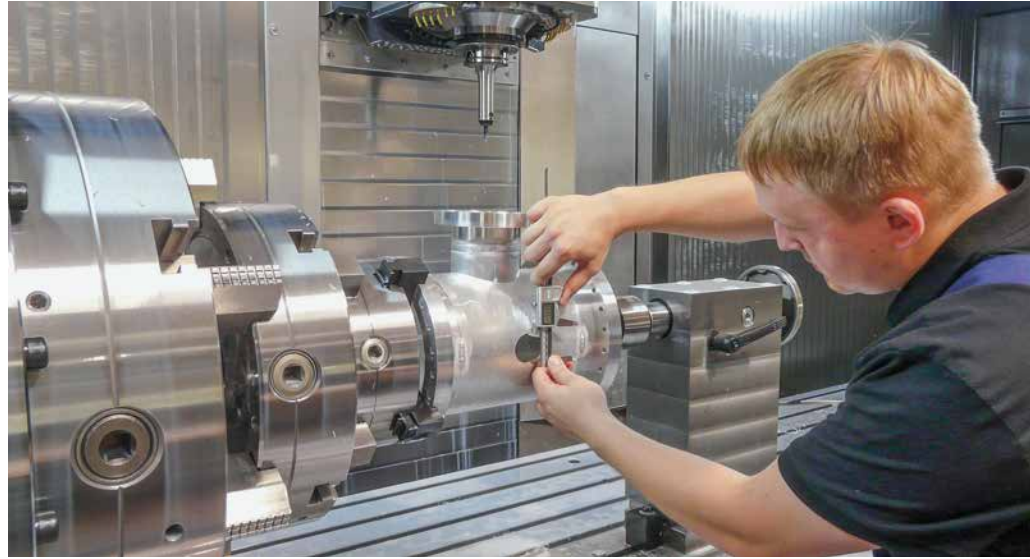
Does the diameter of the hole meet the specifications? A Vacom operator during a quality inspection.
